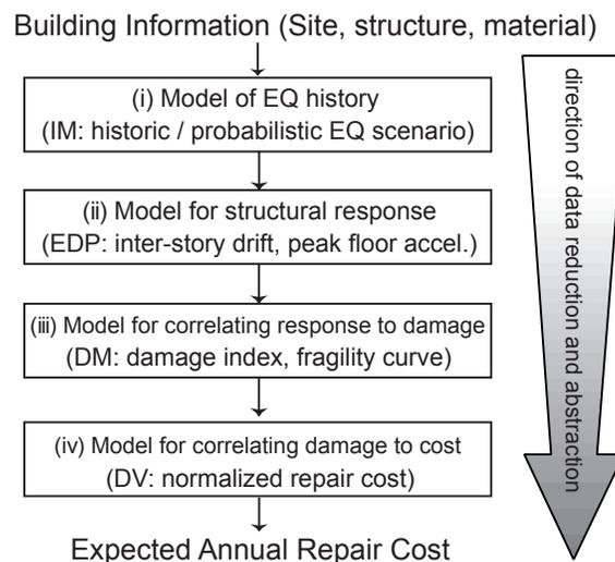
Figure 1. Layered expression of models for the process of estimation of the life cycle cost
