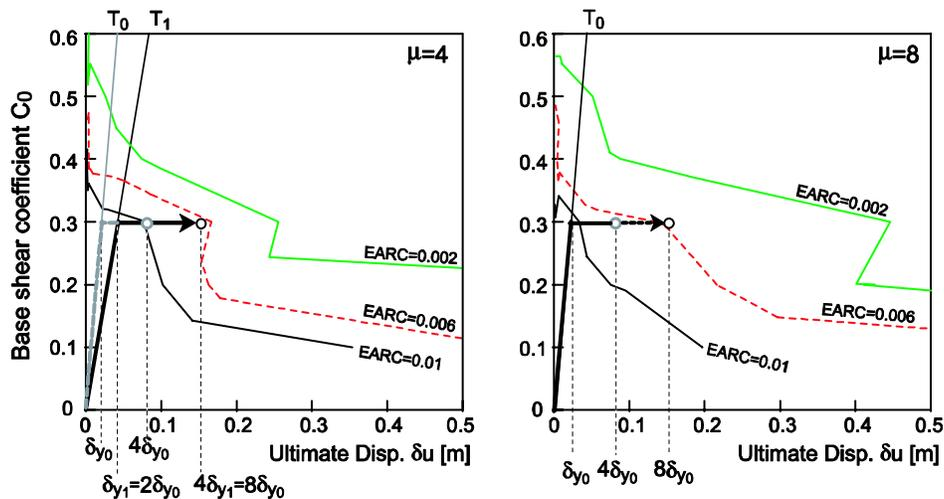
(b) In the case of upgrading a displacement capacity
