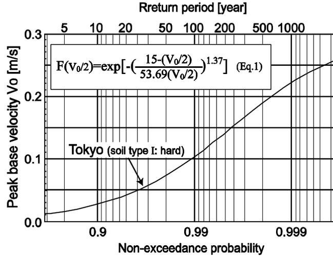
Figure 2. Seismic hazard curve at Tokyo
