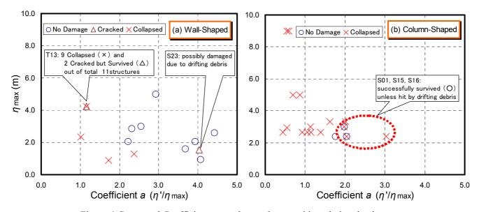
Figure 4 Computed Coefficient a vs. observed tsunami inundation depth  $\eta_{\text{max}}$  (Numerals in the figure denote ID Nos. in Table 1)
