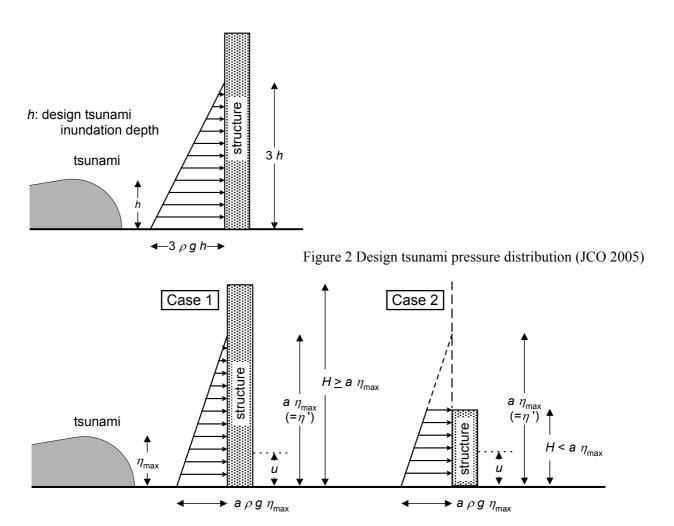
Figure 3 Tsunami inundation depth  $\eta_{\text{max}}$ , building height H, and tsunami pressure distribution  $p_x$  (Nakano 2007)
